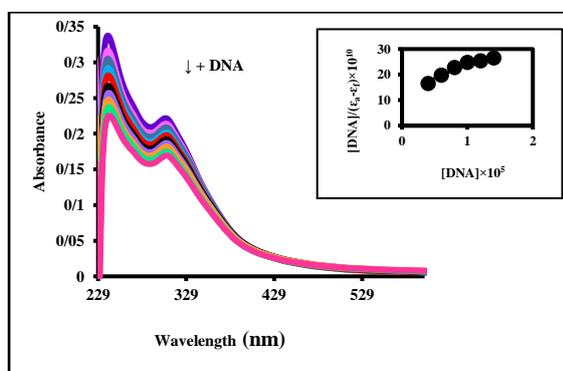
**Fig. 4.** Variations in the electronic spectra of complex (**A**) during the titration with different concentrations of the deoxyribonucleic acid.
