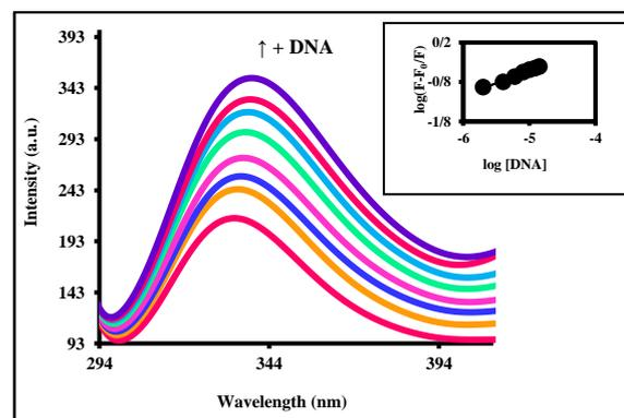
**Fig. 7.** Variations in the fluorescence spectra of complex (**B**) ( $\lambda_{\text{ex}}=258$ ) with increasing concentrations of the deoxyribonucleic acid.
