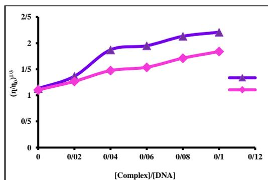
Fig. 10. Viscosity changes for the interaction of DNA and A and B complexes.
