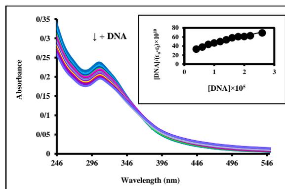
**Fig. 5.** Variations in the electronic spectra of complex (**B**) during the titration with different concentrations of the deoxyribonucleic acid.
