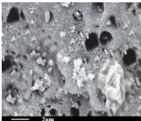
Fig. 3 SEM image of the activated carbon supported iron particles
