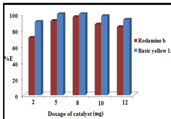
**Fig.8.** Effect of catalyst dosage on degradation efficiencies. Experimental conditions: 100 mL mixture of two dye with concentrations of 12 and 7 mgL<sup>-1</sup> for RB and BY13, respectively, pH 5.5, irradiation time of 60 min.
