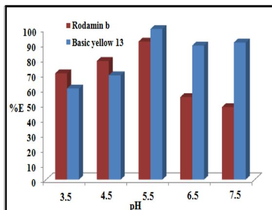
**Fig.6.** Effect of pH on photo-degradation of RB and BY13. Conditions: 100 mL mixture of two dyes with concentrations of 12 and 7 mgL<sup>-1</sup> for RB and BY13, respectively; catalyst dosage, 5 mg; and irradiation time of 60 min.
