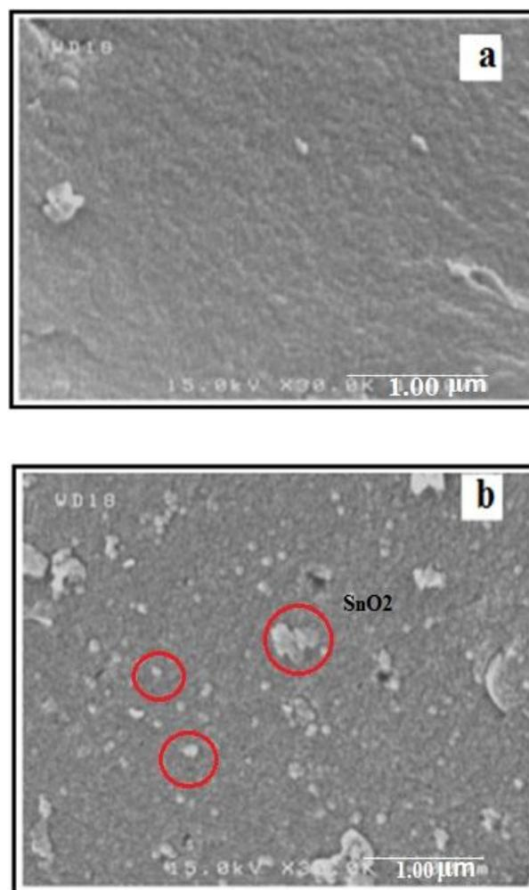
Fig.4. SEM images for (a) AC and (b)SnO<sub>2</sub>/AC.
