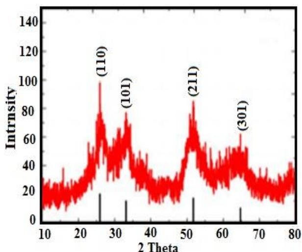
Fig.3. XRD pattern for SnO<sub>2</sub>/AC
