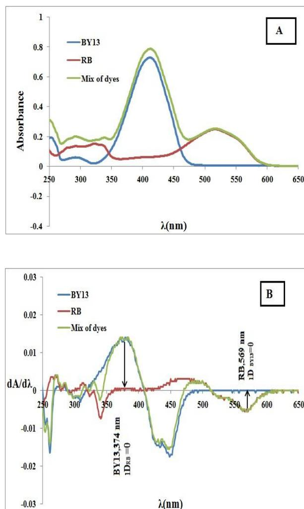
**Fig.1.** (A) Zero-order absorption spectra and (B) first-order absorption spectra for BY13 and RB in single and binary dye solutions, respectively.
