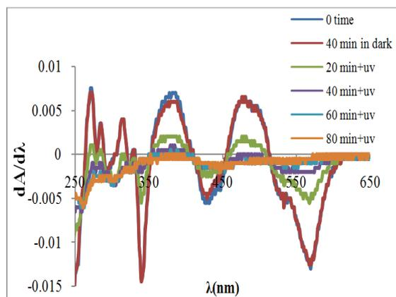
**Fig.5.** First-order absorption spectra for MO solution as a function of UV light exposition time. Conditions: 100 mL of binary solution, 12.0 mg L<sup>-1</sup> of RB and 7 mg L<sup>-1</sup> of BY13; catalyst dosage, 5 mg; and pH 5.5.
