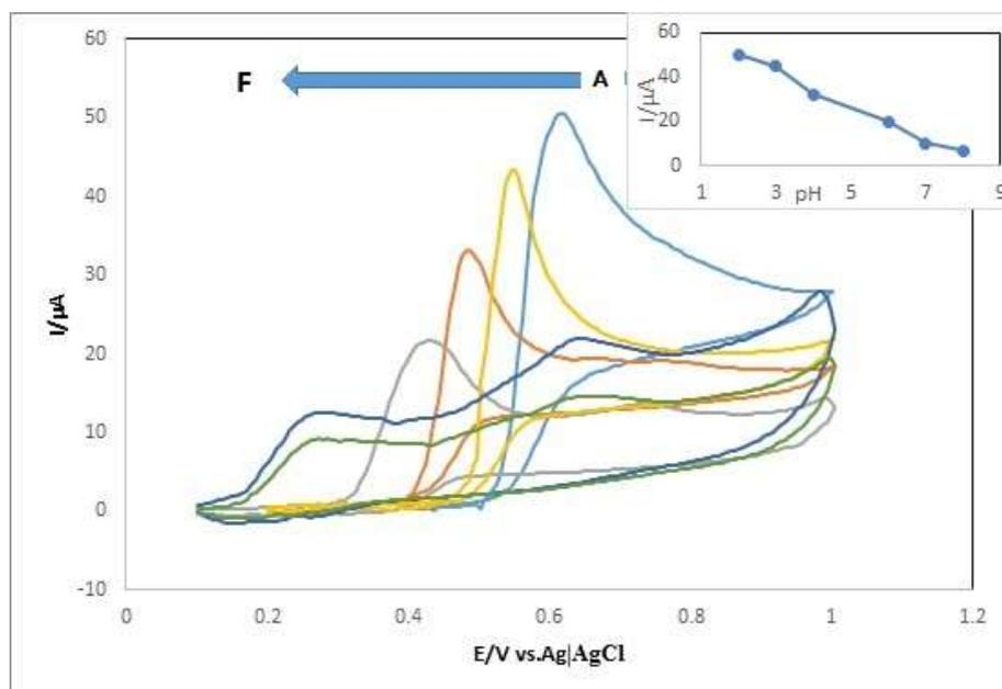
**Fig.6.** Effect of solution pH on the oxidation of 1000  $\mu\text{M}$  ENT at MWCNTs-CPE; scan rate 100 mV/s. pH=A) 2.0, B)3, C)4, D)6, E)7 and F)8. The inset: the linear relationship between pH and I.
