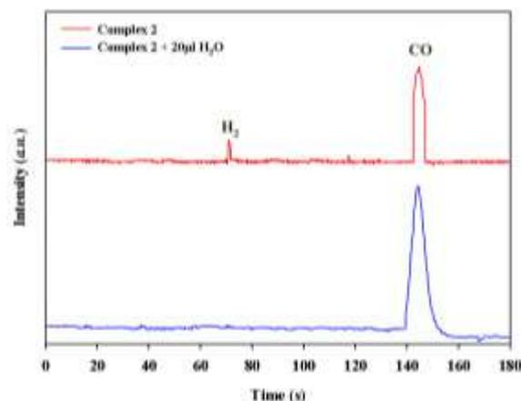
**Fig. 6.** GC analysis of a headspace sample of **2** after 1h electrolysis in absence and presence of 20  $\mu$ l H<sub>2</sub>O.
