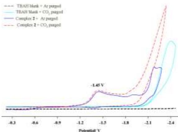
**Fig. 5.** Cyclic voltammograms of **2** in DMF under an Ar (blue) and CO<sub>2</sub> (red) atmosphere. SR = 100 mV/s.
