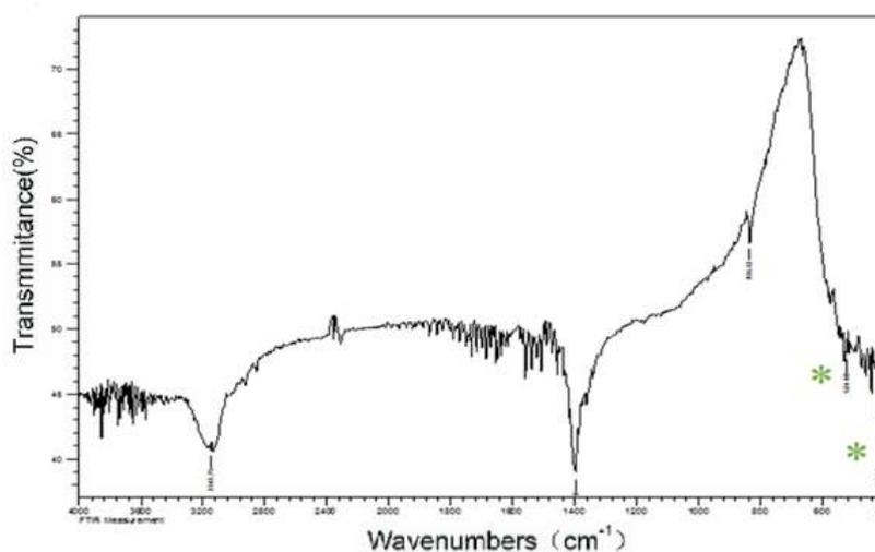
Fig. 2. FT-IR analysis of as-synthesized CuO/CoFe<sub>2</sub>O<sub>4</sub> nanoparticle.
