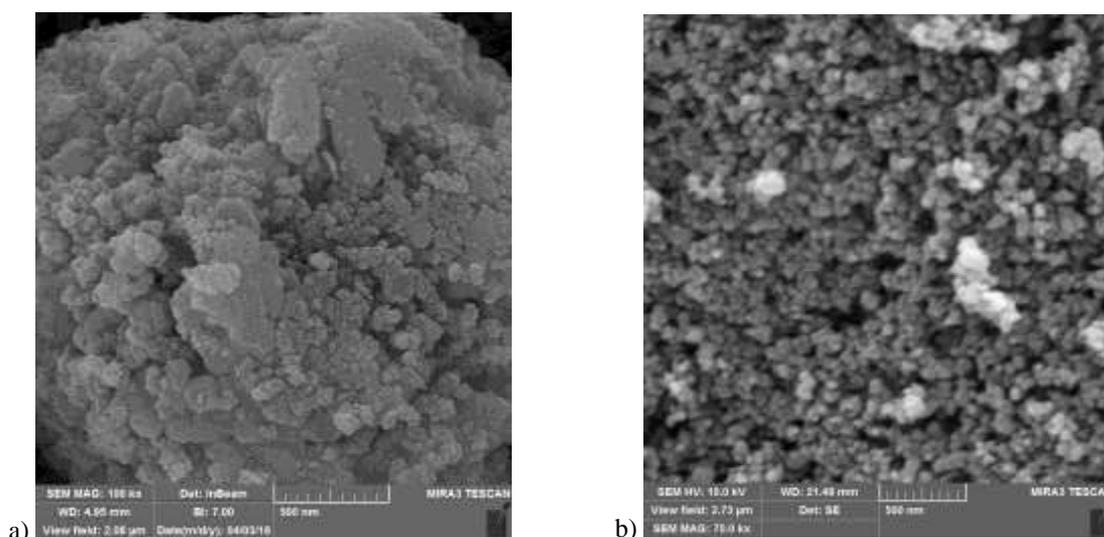
Fig. 4. Fe-SEM image of a) as-synthesized CuO/CoFe<sub>2</sub>O<sub>4</sub>, b) as-received CuO nanoparticle.
