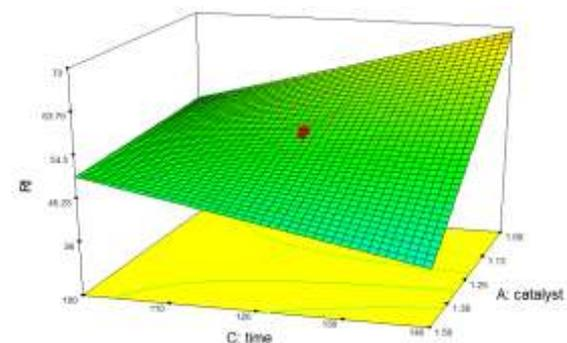
Fig. 8. Effect of catalyst dosage and irradiation time on degradation efficiency.
