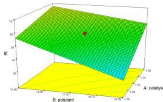
Fig. 7. Effect of catalyst dosage and pollutant concentration on degradation efficiency.
