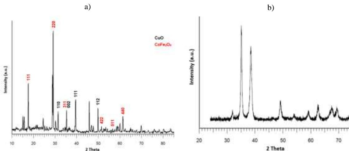
Fig. 1 XRD pattern of a) as-synthesized CuO/CoFe<sub>2</sub>O<sub>4</sub> nanoparticle, b) as-received CuO nanoparticle.
