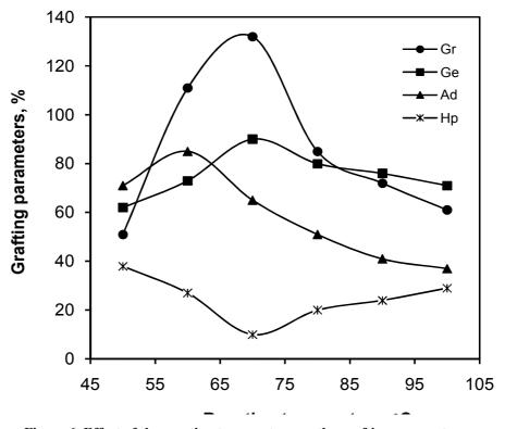
Figure 6. Effect of the reaction temperature on the grafting parameters. Reaction conditions: kC 4 wt%, KPS 0.013 mol/L, AM 0.84 mol/L, time 90 min.
