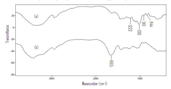
Figure 2. FTIR spectra of kC (a) and graft copolymer, kC-g-PAM (b).
