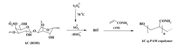
Scheme 1. A brief proposed mechanism for KPS-induced grafting of poly(acrylamide) onto kappa-carrageenan.
