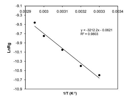
Figure 7. Plot of LnRg versus 1/T for estimating the activation energy of the graft polymerization reaction.
