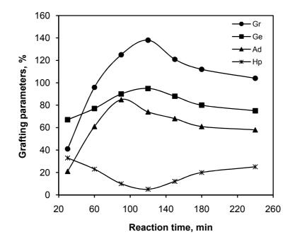
Figure 8. Effect of the reaction time on the grafting parameters. Reaction conditions: kC 4 wt%, KPS 0.013 mol/L, AM 0.84 mol/L, temperature 70°C.
