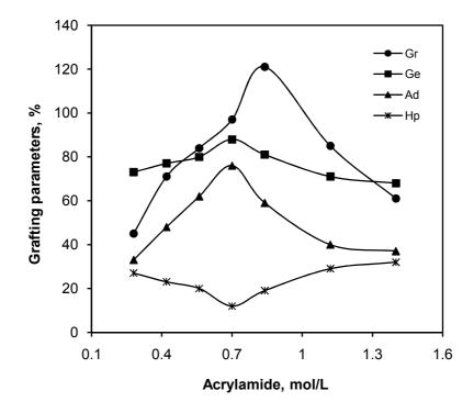
Figure 5. Effect of the monomer concentration on the grafting parameters. Reaction conditions: kC 4 wt%, KPS 0.013 mol/L, temperature 60°C, time 90 min.
