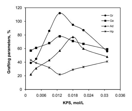
Figure 4. Effect of initiator concentration on the grafting parameters. Reaction conditions: kC 4 wt%, AM 0.7 mol/L, temperature 60°C, time 90 min.
