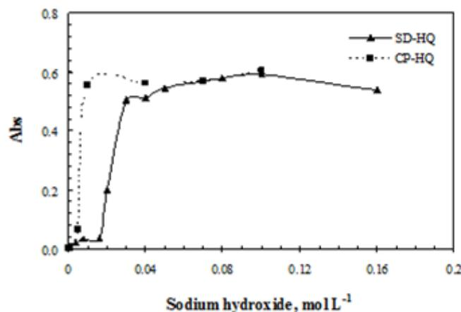
mL solutions containing 10 µg nitrite, SD 1.0 mmol L<sup>-1</sup>, HQ 4.0 mmol L<sup>-1</sup>, hydrochloric acid 0.005 mol L<sup>-1</sup>. Condition for CP-HQ system: 10.0 mL solutions containing 10 µg nitrite, CP 0.5 mmol L<sup>-1</sup>, HQ 1.0 mmol L<sup>-1</sup>, hydrochloric acid 0.008 mol L<sup>-1</sup> and SDS 1.0% (wt/v).
