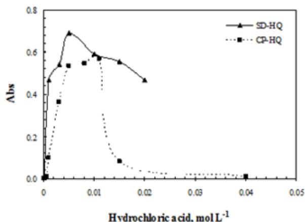
procedures. Condition for SD-HQ system: 10.0 mL solutions containing 10 µg nitrite, SD 1.0 mmol L<sup>-1</sup>, HQ 4.0 mmol L<sup>-1</sup>, sodium hydroxide 0.04 mol L<sup>-1</sup>. Condition for CP-HQ system: 10.0 mL solutions containing 10 µg nitrite, CP 0.5 mmol L<sup>-1</sup>, HQ 1.0 mmol L<sup>-1</sup>, sodium hydroxide 0.01 mol L<sup>-1</sup> and SDS 1.0% (wt/v).
