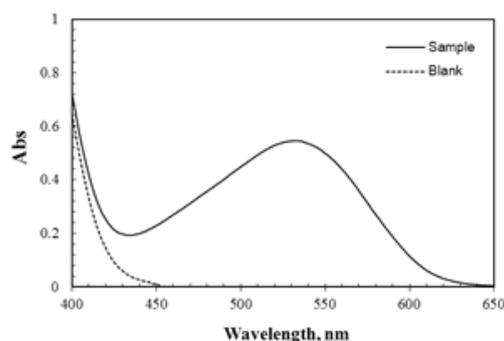
Figure 2. Absorbance spectra blank and 10 µg nitrite containing sample solution. Condition: 10.0 mL solutions containing hydrochloric acid 0.005 mol L<sup>-1</sup>, CP 0.5 mmol L<sup>-1</sup>, HQ 1.0 mmol L<sup>-1</sup>, sodium hydroxide 0.10 mol L<sup>-1</sup> and SDS 1.0% (wt/v).
