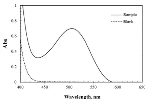
Figure 1. Absorbance spectra of blank and 10 µg nitrite containing sample solution. Condition: 10.0 mL solutions containing hydrochloric acid 0.01 mol L<sup>-1</sup>, SD 1.0 mmol L<sup>-1</sup>, HQ 4.0 mmol L<sup>-1</sup> and sodium hydroxide 0.10 mol L<sup>-1</sup>.
