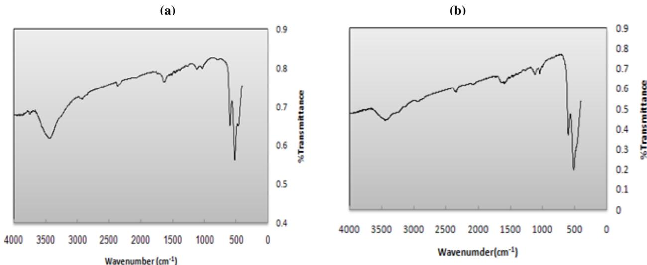
Figure. 2. FT-IR spectra of (a) CuO and (b) Sn doped CuO nanoparticles
