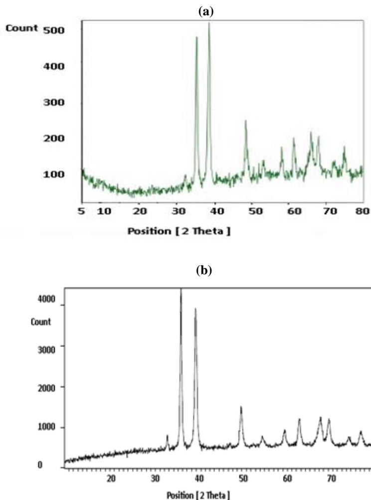
Figure 1. XRD pattern of (a) CuO and (b) Sn doped CuO nanoparticles.
