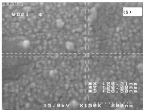
Figure.3.SEM image of Sn doped CuO nanoparticles
