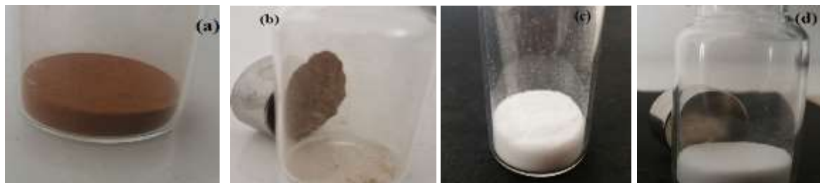
Figure 1. (a) Perlite/ \text{Fe}_3\text{O}_4 magnetic nanocatalyst (b) Perlite/ \text{Fe}_3\text{O}_4 magnetic nanocatalyst with an external magnet, (c) perlite (d) perlite with an external magnet
