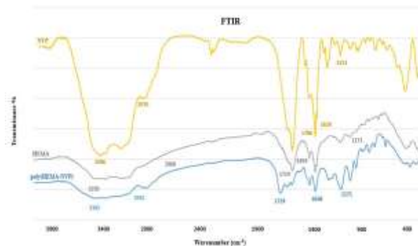
Fig. 2. FT-IR spectra of poly (HEMA-co-NVP) hydrogel, HEMA, and NVP.
